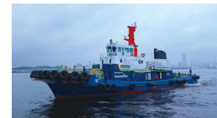
Tugboat equipped with ammonia combustion engine
