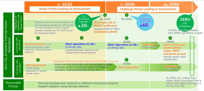
This roadmap will be gradually developed in greater detail based on relevant conditions such as government policies. JERA will revise the roadmap when relevant conditions change significantly. \*The use of  $CO_2$ -free LNG is also being considered.
