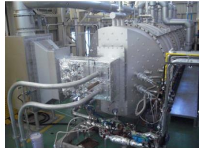
Ammonia combustion test facility (0.5 ton/h combustion test furnace) Source: MHI Press Release ( https://www.mhi.com/news/23112801.html )
